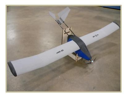
The EP-3000 is a tough, survivable, fixed-wing sensor platform designed for missions covering long loiter times. Emphasis has been placed on stability, ruggedness and payload capacity. Principal applications include: precision agriculture services, public utilities applications, emergency response, and search and rescue missions. The EP-3000 is a custom designed aircraft that can be tailored to user requirements.
